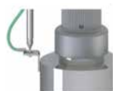
Fig. 12 - Ground Screw Connection
