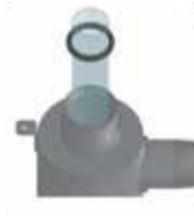
Fig. 6 - Quartz Sleeve Installation
